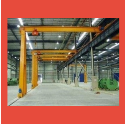
Semi Gantry Cranes
