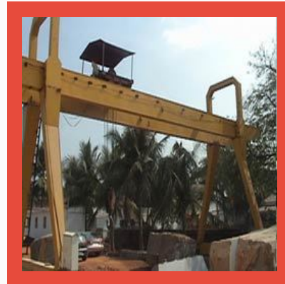
Semi Goliath Cranes
