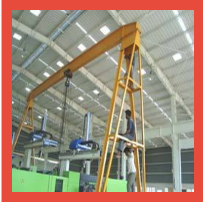
A Frame Cranes
