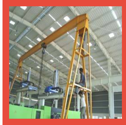
A Frame Cranes
